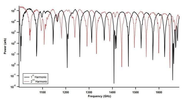
The figure (above) illustrates a single scan of laboratory air without any processing (smoothing) or averaging. The phase modulation technique allows the detection of the first and second harmonics as shown in the plot above: summing the harmonics results in the fringe free spectrum shown below. No secondary processing was performed on the data.
